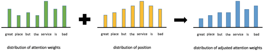
Fig. 1. The illustration of how position distribution adjusts attention weight distribution. The green, yellow and blue represent original attention weight distribution, position distribution, and adjusted attention weight distribution respectively. The target is “ service ”. (Color figure online)
